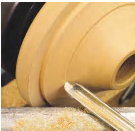
▲ Pic.13 Rough the base to shape with some pull cuts using the long-grind bowl gouge before switching to the micro bevel tool and using a fine finishing push cut
